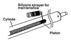
4 Wipe the dust or dirt on the ring. If the screw is loose, tighten it.
